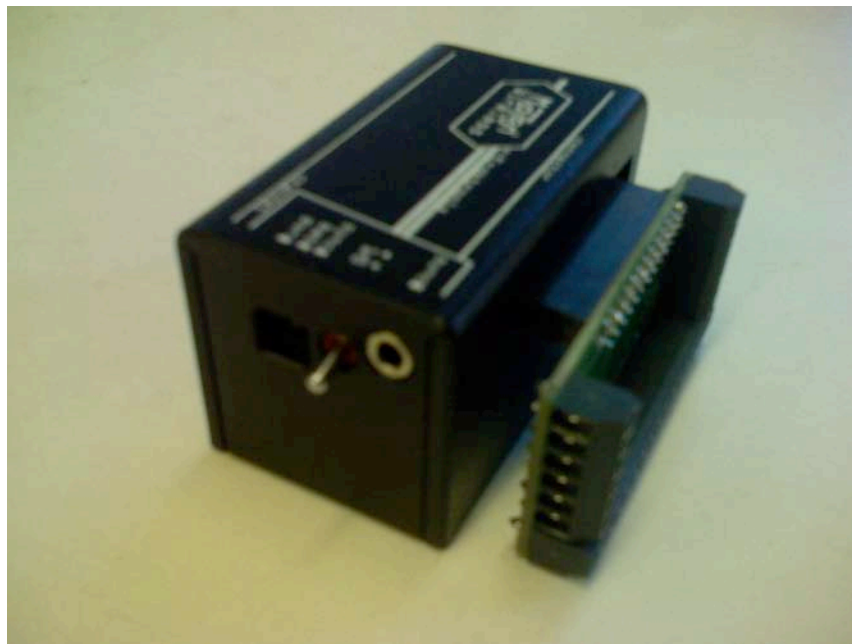
Figure 5: How to orient connector boards
